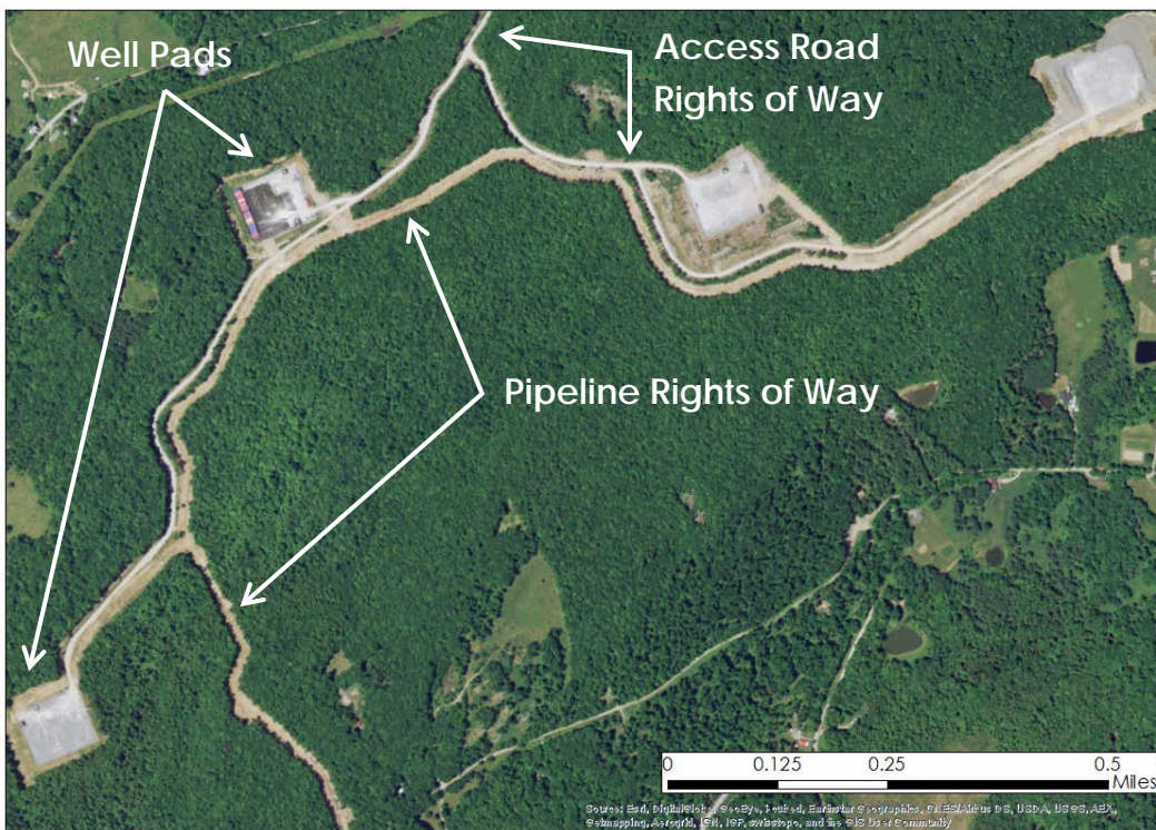
Figure 5. Imagery depicting several existing well pads and associated infrastructure rights-of-way in Susquehanna County, PA. This provides an example of the potential footprint associated with natural gas development.
